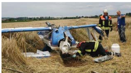
Top: With insufficient height to recover from the vertical, the Zlin-142 impacted within the airport boundary (Index).
