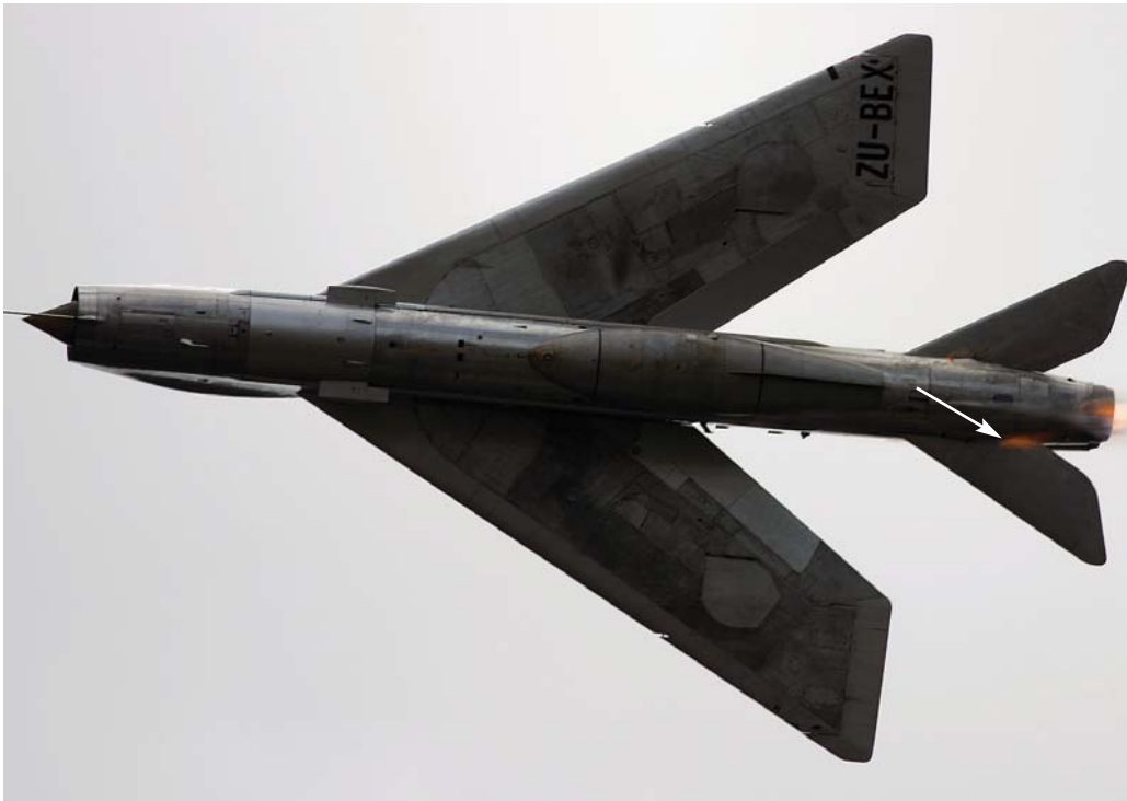
The ill-fated English Electric Lightning seen flying its demonstration shortly before the pilot reported hydraulic failure. The fire in the tail pipe (arrowed) which grew rapidly is thought to have caused the total failure of the aircraft's hydraulic systems causing the pilot to lose control. He was unable to eject because of an ejection seat failure (see also Page 71).
